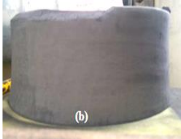
Fig 3: Roll pressed after adopting vibrational method while powder milling
