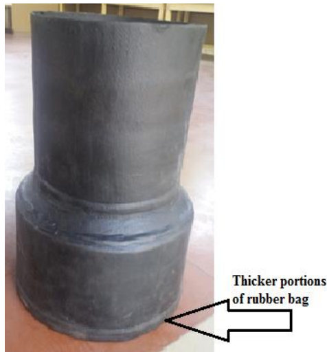
Fig-6: More thicker portions observed near bottom of rubber bag
